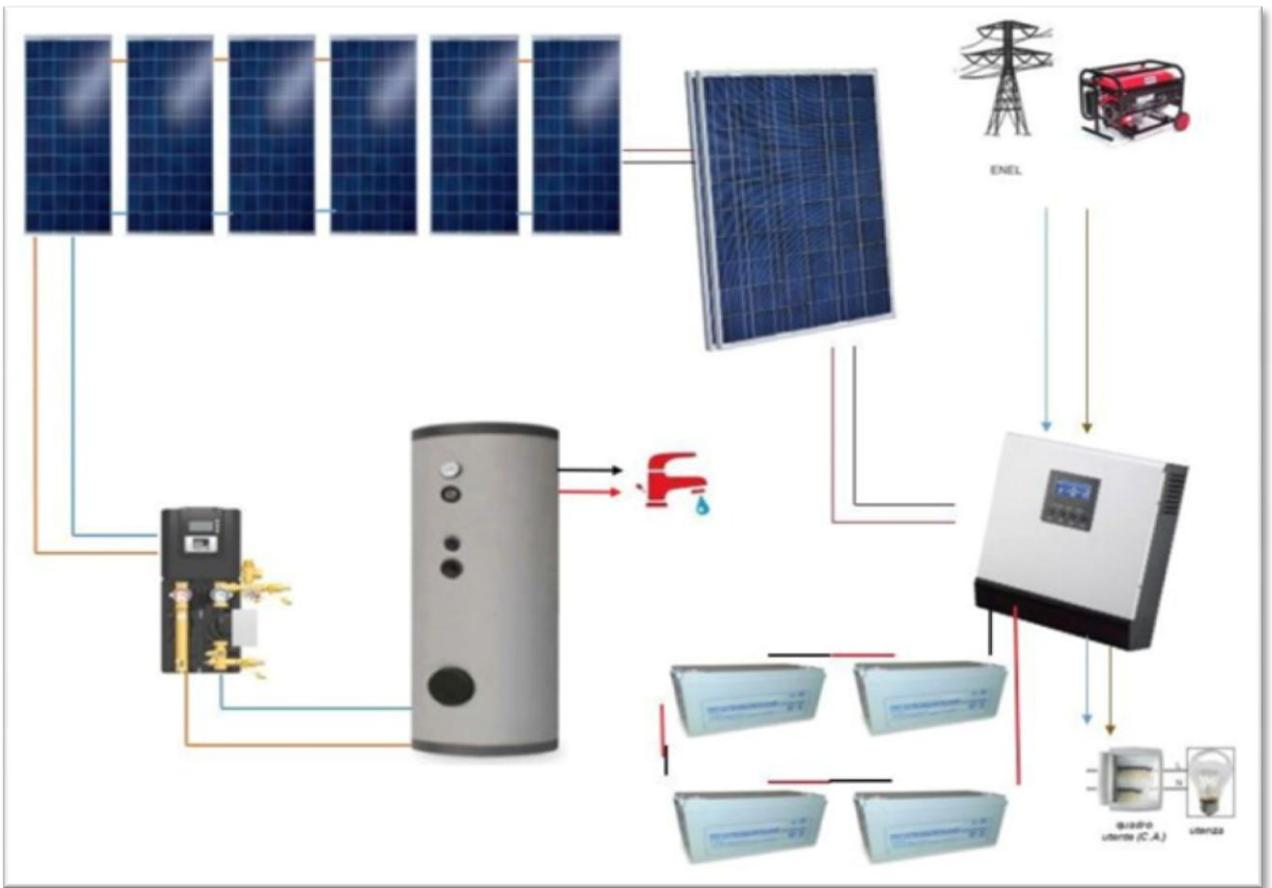
*Photovoltaic system complete with panels, batteries, inverters and solar thermal system for the production of hot water for the production and washing of dairy products.*
